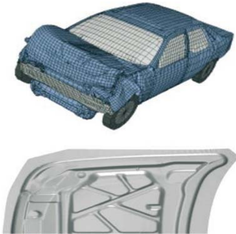
Fig. 3. Hood frame deformation in a frontal impact scenario.
