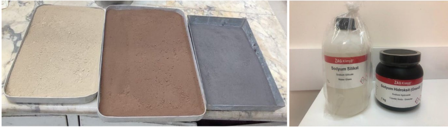
Fig. 1 Clay, Karacadağ red scoria (KS), and RHA raw materials, sodium silicate ( \text{Na}_2\text{SiO}_3 ) and NaOH alkali activators
