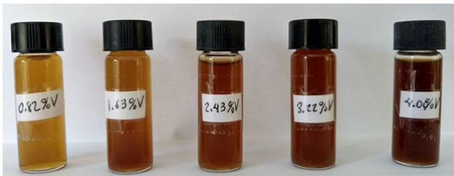
Fig. 1 Preparation of graphene oxide (GO) for different concentrations 0.82 %V, 1.63 %V, 2.43 %V, and 3.22 %V, 4 %V by the method of Hummers [19]
