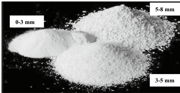
Fig. 1 Expanded perlite aggregates sized as 0–3 mm, 3–5 mm, 5–8 mm
