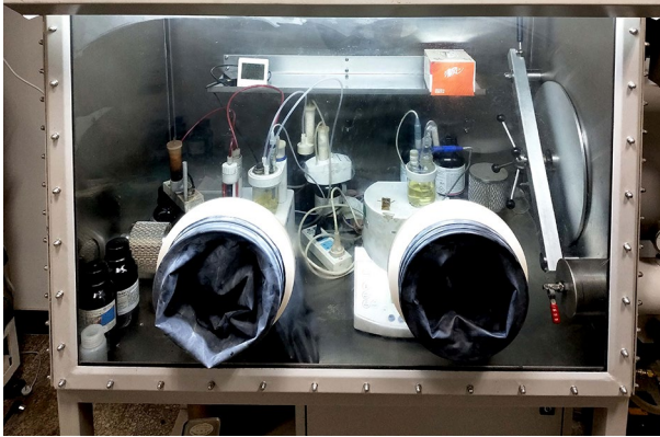
Fig. 1 Karl Fischer coulometric and volumetric titrators in the glove box
