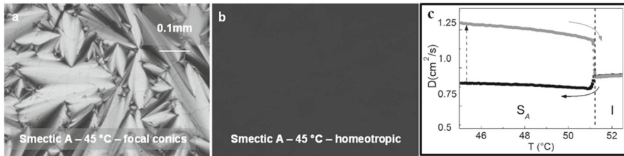
Fig. 3 (a) Focal conic texture in the smectic A phase of 10CB liquid crystal; (b) non-birefringent polarization microscopy pattern obtained in homeotropically aligned smectic A phase; (c) thermal diffusivity values corresponding to situation in (a) (black symbols) and in (b) (gray symbols)
