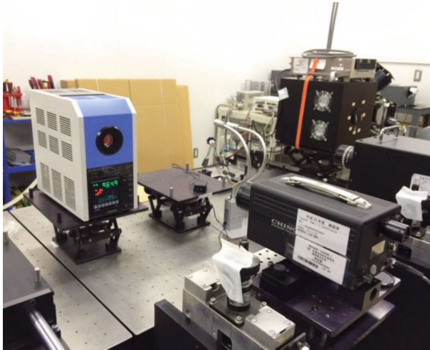
Fig. 2 Arrangement of the fixed-point sources and the radiation thermometers within the laboratory
