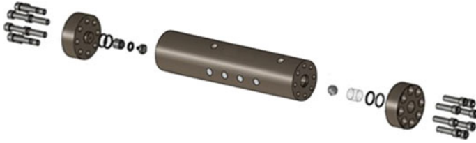
Fig. 2 Expanded view of the windowed variable-volume rolling-ball viscometer
