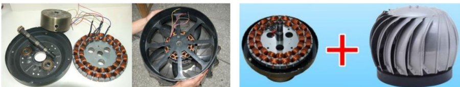
Fig. 6 Students disconnected ceiling fan wires and put them together with a ventilation ball to create a roof ventilator for electricity generation
