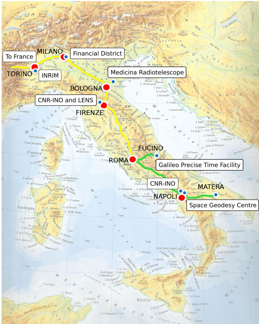
Fig. 7 Present day dissemination of the fiber link in Italy, in yellow the already working link, and in green the upcoming connections
