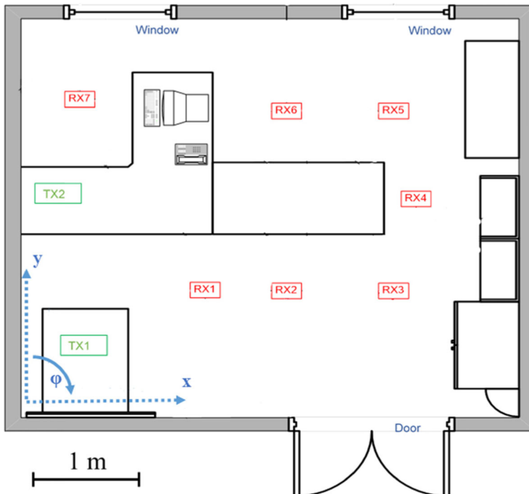
Fig. 1 2D map of the indoor office. TXs in green and RXs in red. Some details in blue
