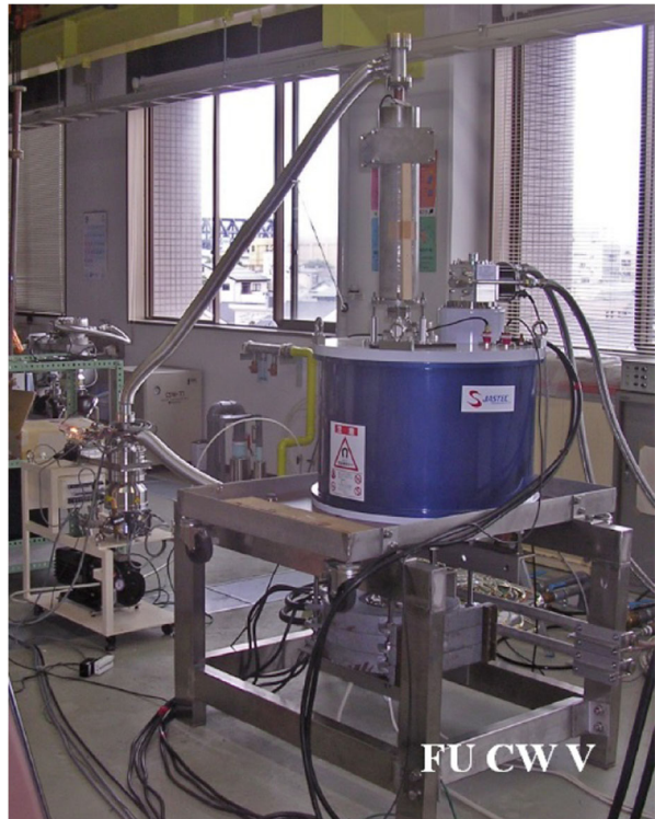
Fig. 5 Gyrotron FU CW V with an 8-T superconducting magnet
