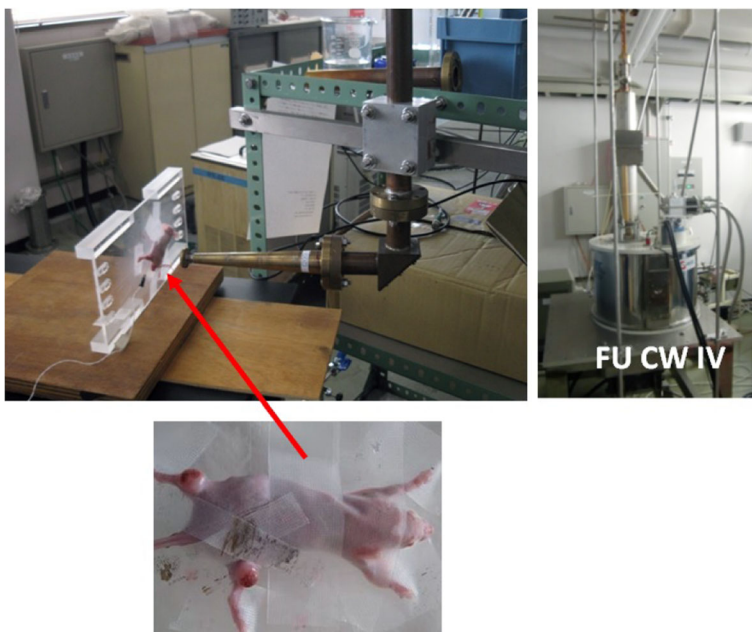
Fig. 19 Experimental setup for in vivo irradiation of animals with cancerous tumors by sub-THz radiation: radiation source FU CW IV ( right panel ) and the irradiation stage ( left panel )
