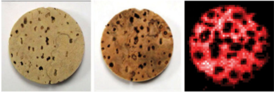
Figure 3 Evaluation of cork enclosures by terahertz imaging taken from [115]
