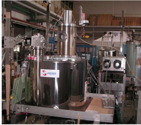
Fig. 2 Photograph of Gyrotron FU CW GII mounted on an 8 T superconducting magnet
