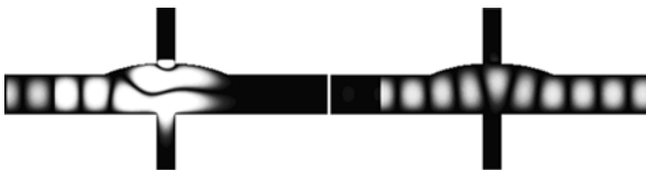
Fig. 2 Electric field plots for 70 GHz microwave; left—laser off and the switch closed, right—laser on and the switch open.
