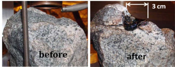
Fig. 5 Before and after photos of third granite specimen with a non-flat surface showing the peaked ridged surface ablated away by the 28 GHz gyrotron beam.
