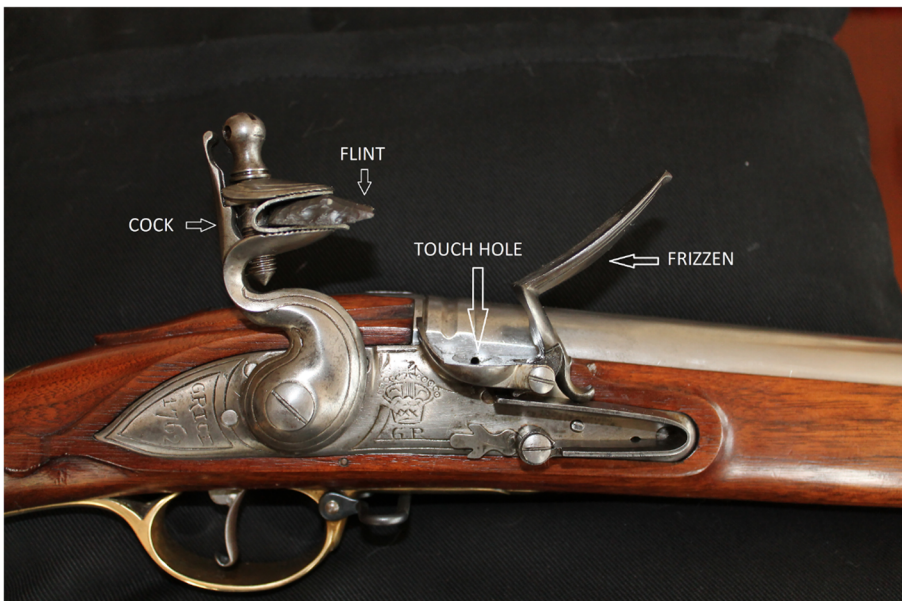
Fig. 1 Flintlock mechanism and terminology
