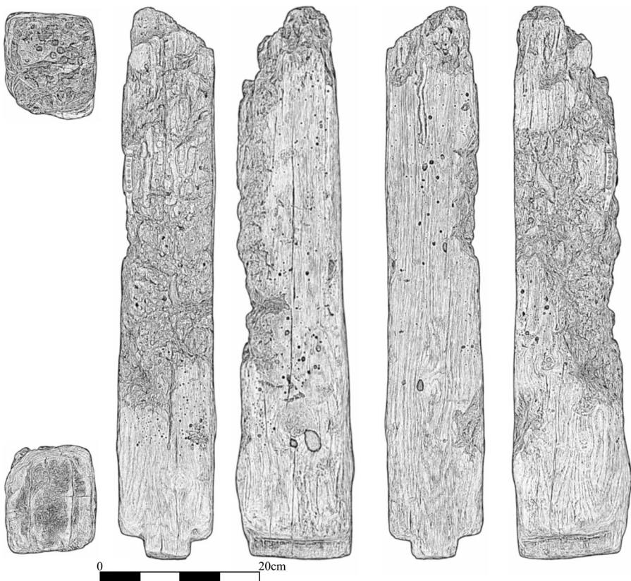
Fig. 7 Deck stanchion originally located forward of the mainmast step. (Drawing by Author)
