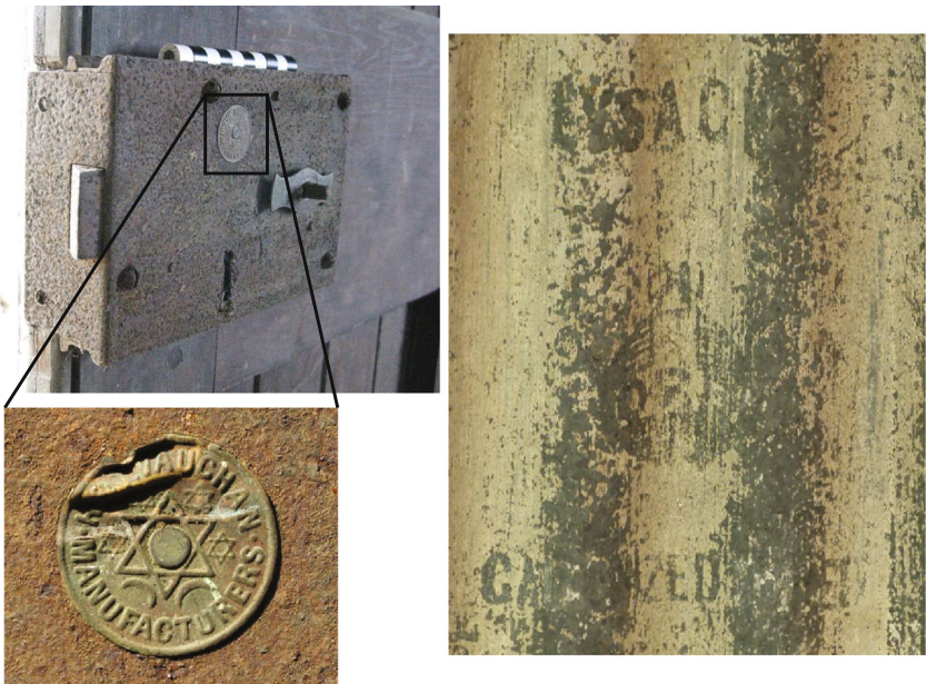
Fig. 8 Artifacts of Empire: H & T Vaughan Manufacturers Draw Back Lock, from Willenhall, England (left), and Lysaght “Orb” galvanized roofing iron, probably from Bristol, England
