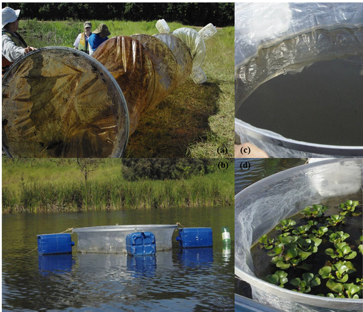
Fig. 1 Experimental enclosures introduced in the pelagic zone of the lake. Photographs show how the mesocosms look in various states, such as outside the water after removal. The 1.3 m diameter and 5 m in length can be seen in the picture with
