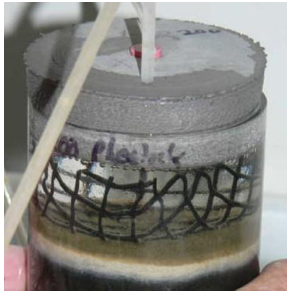
Fig. 1 Assembled incubation chamber showing the position of the cup-shaped 1-cm mesh plastic screen which was fitted between the sediment and the cap on the incubation chamber. The flat bottom of the mesh cup was in contact with the sediment surface
