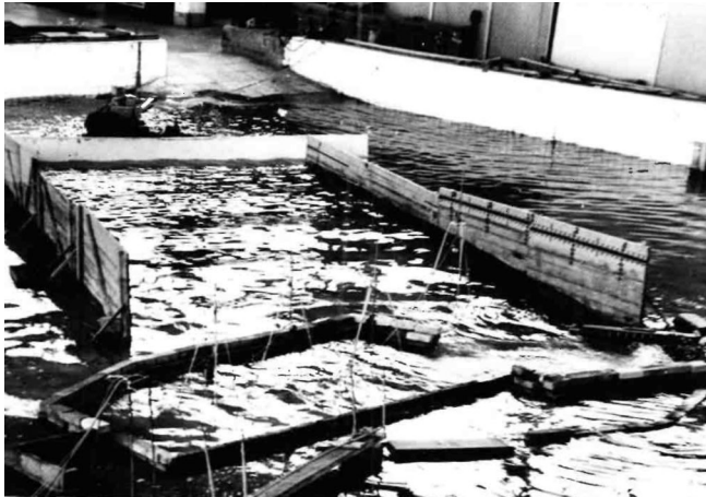
Fig. 2. General view of a model of the port protected by a single pier.
