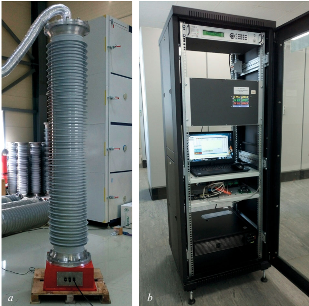
Fig. 3. Layout of a high-voltage primary converter with an optical sensor inside (a) and an electro-optical digital processing unit (b) in a 19-inch rack.
