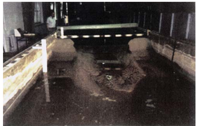
Fig. 5. Shape of breach after termination of experiment.
