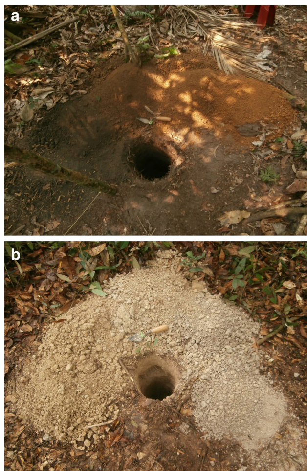
Fig. 5 a Augured posthole by terra firme transect point SU 00. The soil heap farthest to the right represents the most superficial levels; the left one represents the deepest levels. b Augured posthole by riverine forest transect point SU 02. The soil heap farthest to the right represents the most superficial levels; the left one represents the deepest levels
