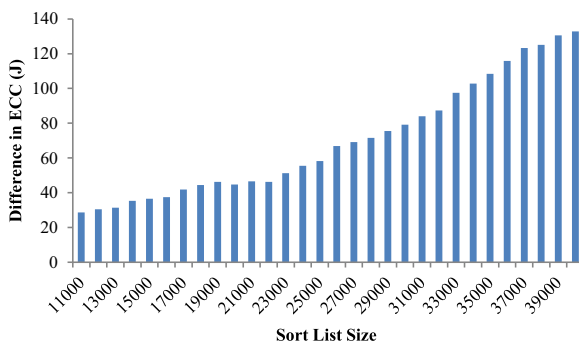
Fig. 6 Difference in ECC of sort service execution on mobile device and traditional computational offloading
