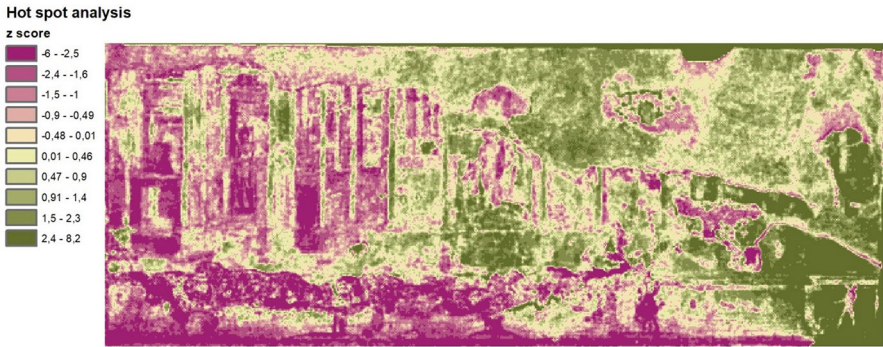
Fig. 7 Hotspot analysis for V raster. Green areas shows the progressive phenomenon of decoloration of the existing pictorial pigments
