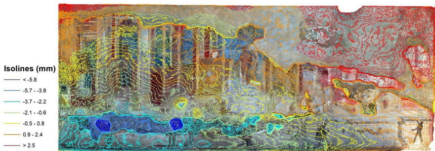
Fig. 10 Contouring derived from DRM. The orange and the cyano classes could reveal areas more at risk
