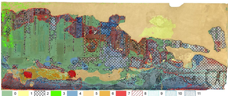
Fig. 14 The final map with decay patterns and risk areas extracted with spatial analysis
