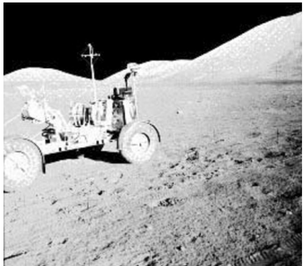
Fig. 1 The surface electrical properties experiment carried out on Apollo 17 used a 3-component vector receiver mounted on the lunar rover and a dual axis multi-frequency dipolar antenna laid out on the surface to sound the subsurface (from Annan 2002)
