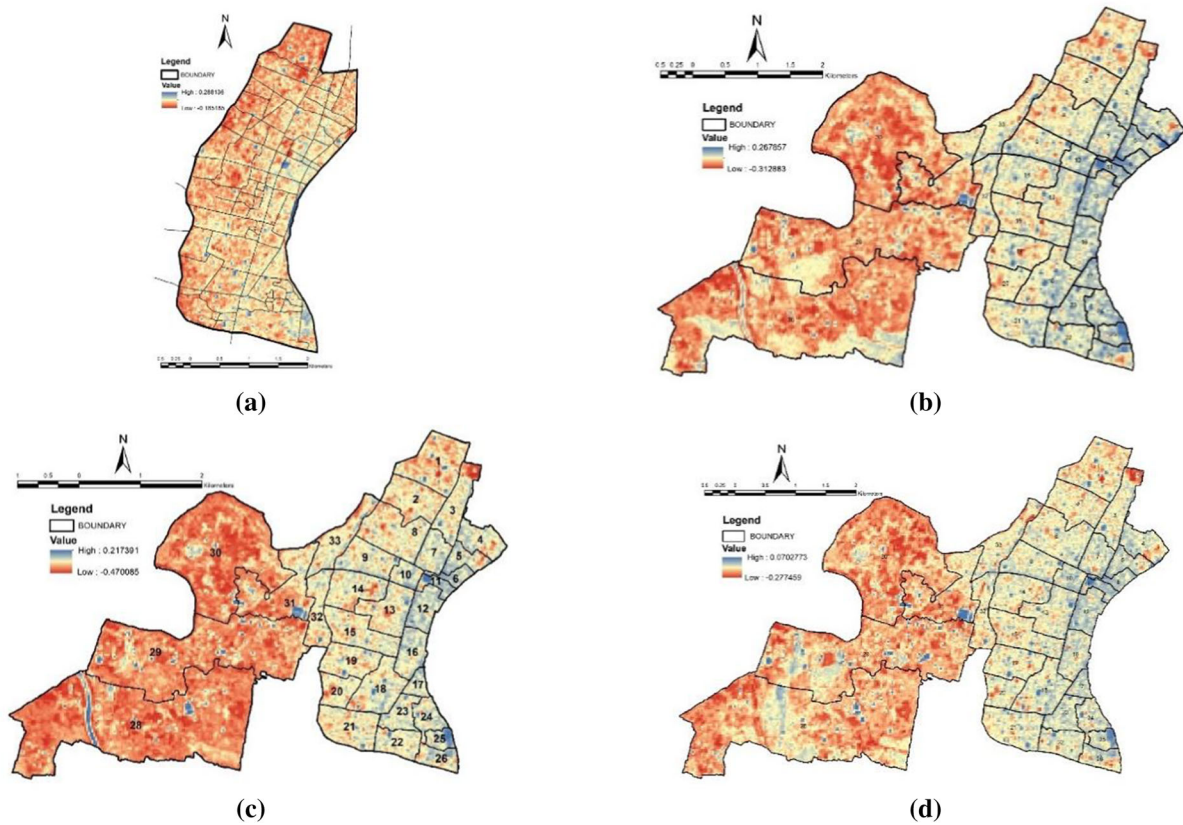
Fig. 5 NDWI derived from Landsat images for the years: (a) 1991; (b) 2001; (c) 2011; (d) 2020
