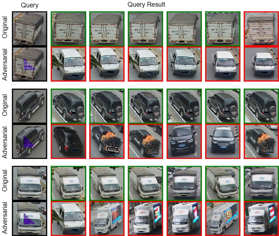
Fig. 5 Examples of attack results on open-VehicleReID on VeRi776 dataset. Green box for correct samples and red for incorrect samples
