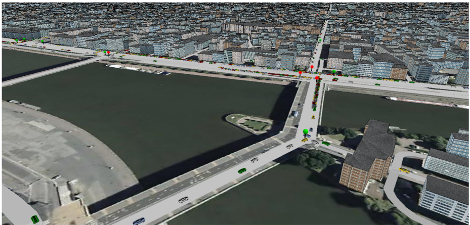
Fig. 6 Example of displays that can be defined with GAMA: used of 3D obj files with textures for cars, a geo-referenced satellite image as background, and a building shapefile with 3D extrusion and textures for buildings
