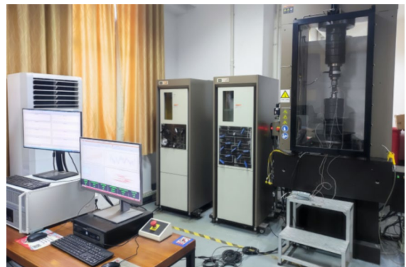
Fig. 2 MTS 815 high rigidity rock mechanics test system
