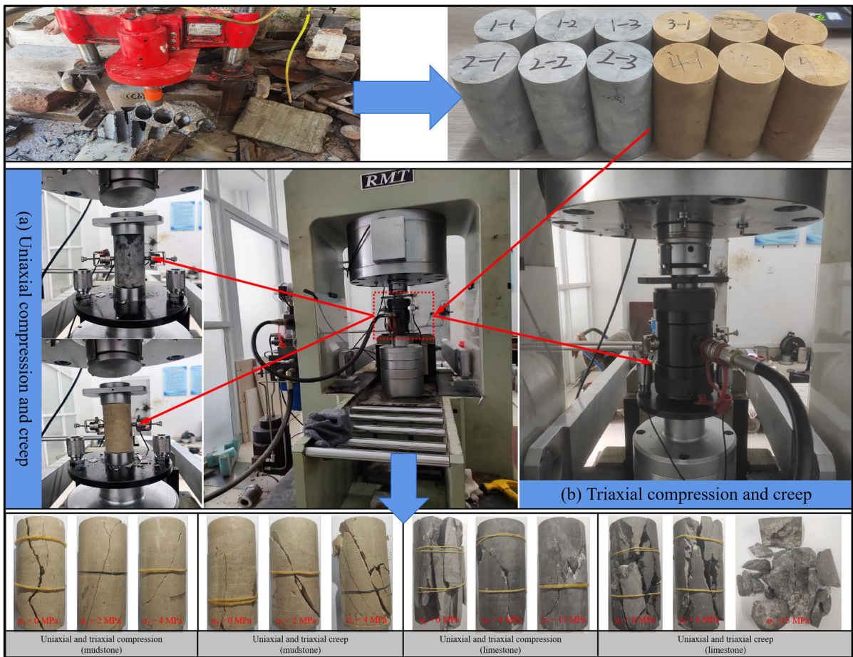
Fig. 4 Test equipment and specimen loading
