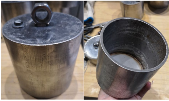
Fig. 1 Bucket foundation scale model
