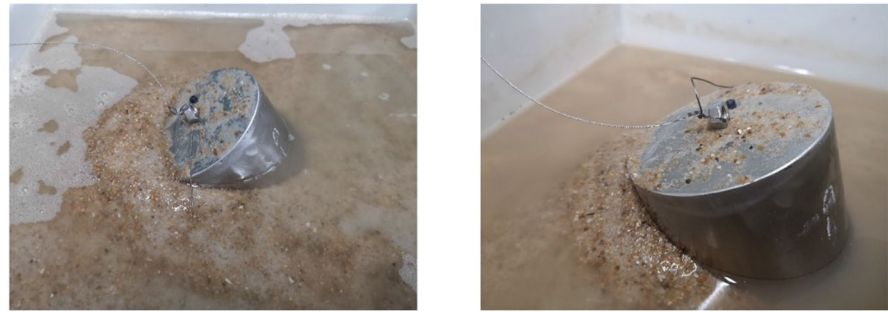
(a) 15° pull-up drawing of bucket foundation (b) 45° pull-up drawing of bucket foundation
