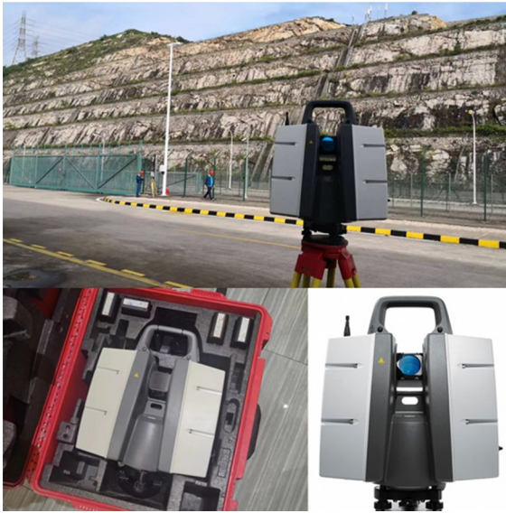
Fig. 18 Photo of the Swiss Leica ScanStationP40 high-speed 3D laser scanner
