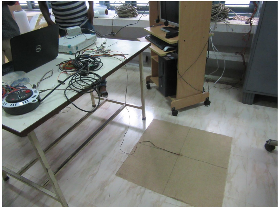
Fig. 11 Testing of strain gauge prior placing into the test tank
