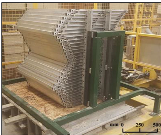
Fig. 3 Flexible Laminar Shear Box (FLSB) developed and built for this study
