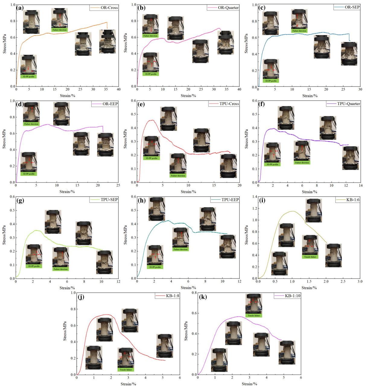
Fig. 10 Failure evolution of CTB specimens: a OR-Cross; b OR-Quarter; c OR-SEP; d OR-EEP; e TPU-Cross; f TPU-Quarter; g TPU-SEP; h TPU-EEP; i KB-1:6; j KB-1:8; k KB-1:10
