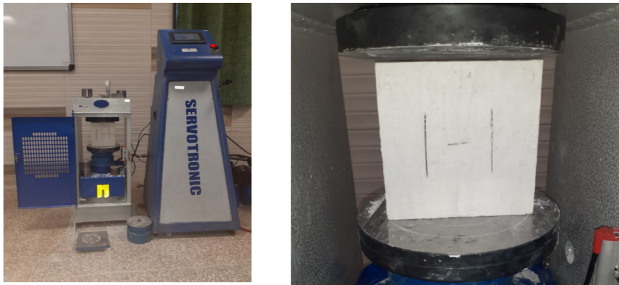
Fig. 6 Specimen placed between the plates of the loading machine
