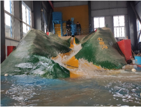
Fig. 6 Measurement of flow velocity of water flow and water-stone flow under various conditions
