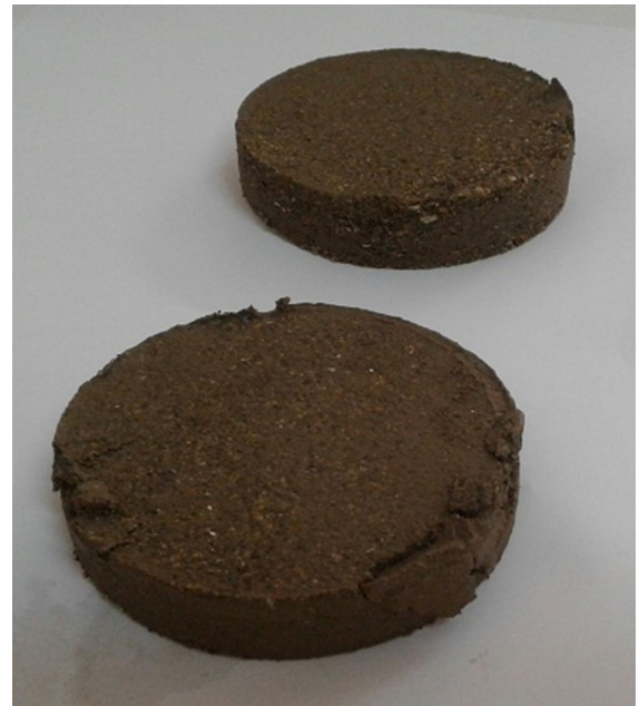
Fig. 3 View of samples after oedometric test
