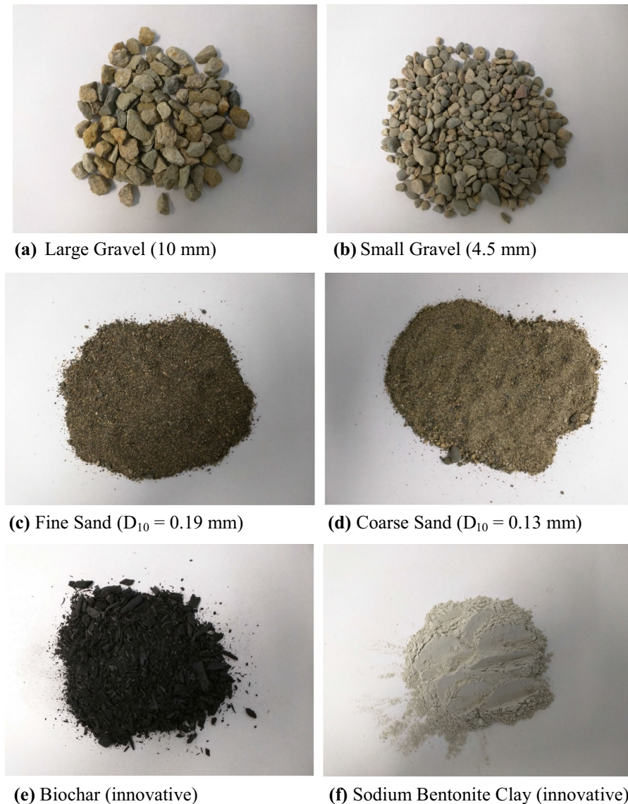
Fig. 1 Common and innovative soil samples that were utilized in the experimenting process
