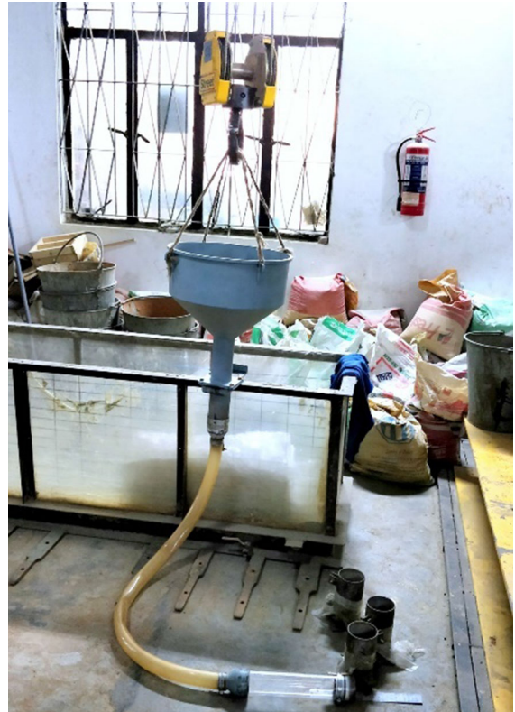
Fig. 3 Portable pluviator for construction of the model wall
