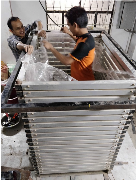
Fig. 2 Membrane is being attached inside the laminar box
