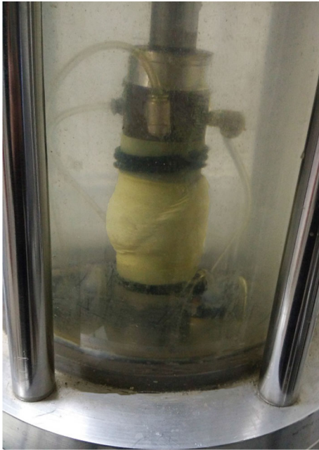
Fig. 17 Failed unsaturated test specimen
