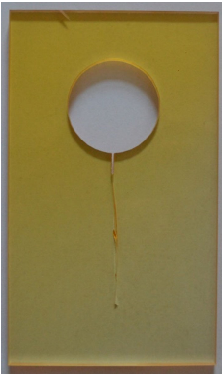
Fig. 7 Crack pattern after the experiment
