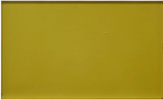
Fig. 4 The epoxy resin plank after solidification and annealing
