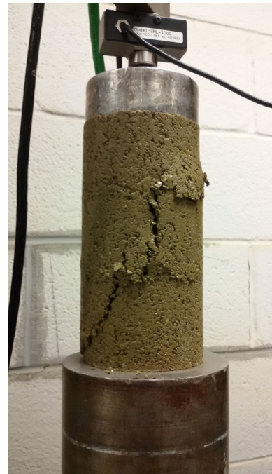
Fig. 6 Typical failed sample from UCS test
