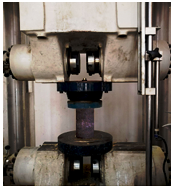
Fig. 4 Uniaxial compression test using the MTS machine
