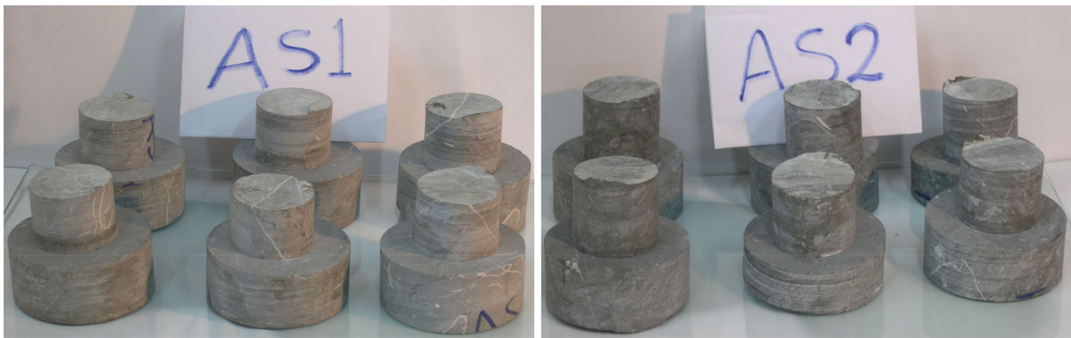
Fig. 1 Some of samples prepared for saw-cut tests with diameter of 54 and 94 mm
