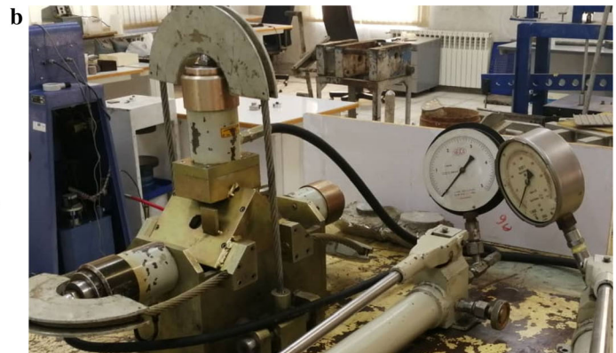
Fig. 4 a Schematic view of the direct shear test apparatus and, b direct shear test apparatus for measuring the basic friction angle
