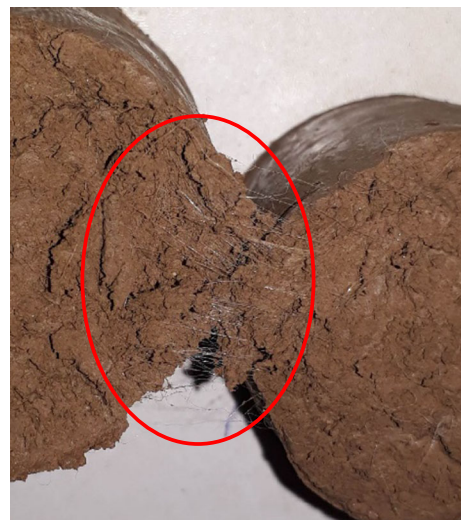
Fig. 1 Fiber-reinforced clay with 0.2% PP fibers
