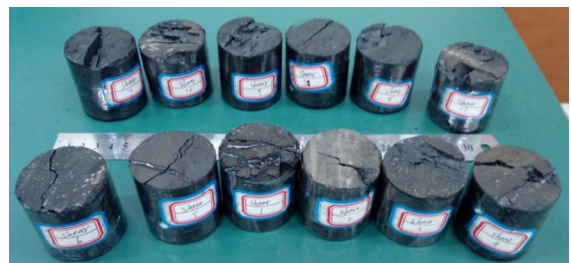
Fig. 4 Single fractured coal samples after shear test
