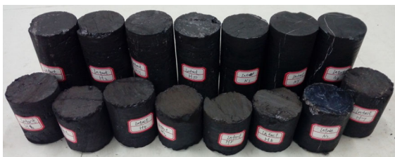
Fig. 3 Raw coal samples
